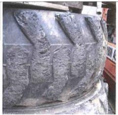
UNACCEPTABLE – Severe tread wear
