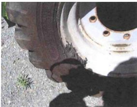
UNACCEPTABLE – Bead damage
