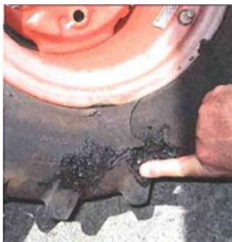
UNACCEPTABLE – Severe side wall damage
