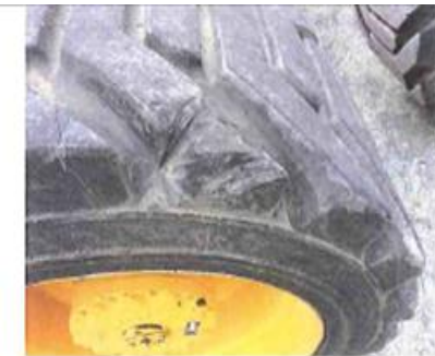
Non-critical – Small amount of tread missing but outer case is not damaged
