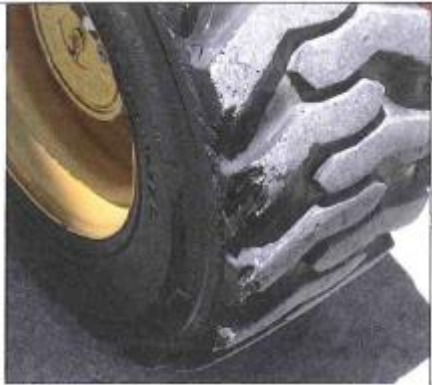
Non Critical – Small amount of tread missing
