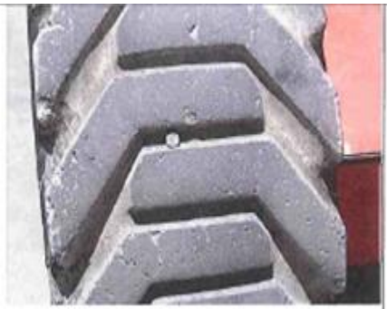
Bolt in tyre – this is not a fault – bolt is used to plug their air hole after filling
