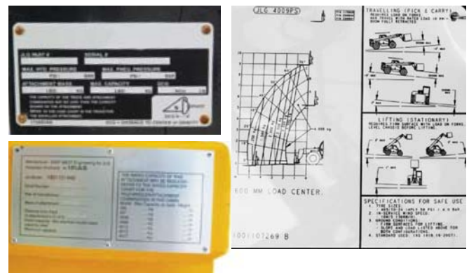
Examples of compliance plates and load charts for telehandlers.
