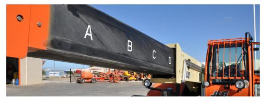
Figure 5: Typical boom length indicator (mechanical)
