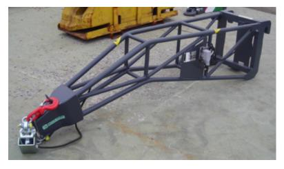
Figure 13: Roof-truss jib
