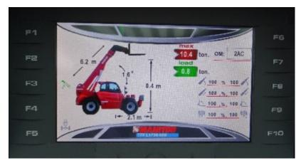
Figure 6: Typical boom length indicator (electronic)
