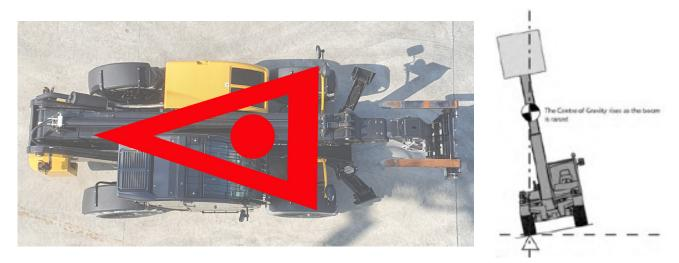
It is important to consider the telehandler stability in three configurations – longitudinal (forwards stability), lateral (side stability) and rearward stability.
