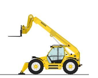
Figure 3: Typical non-slewing telehandler
